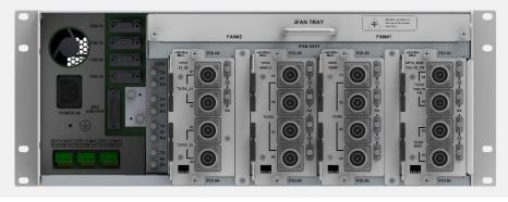
The iBIU receives RF signals from, and sends RF signals to, the base station (BTS) or bi-directional amplifier (BDA). In the iBIU, each signal is independently filtered, attenuated and controlled. The optical modules in the iBIU convert the RF and optical signals and transmits them via fiber to and from the remote units (ROUs).
